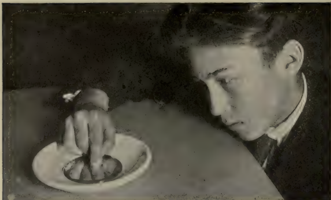
FIG. 23. The mercury does not wet the finger, and as the finger is lifted the mercury does not follow it.
